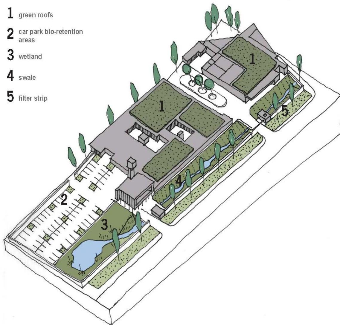
Figure 6.18: Incorporating SuDS on industrial sites
